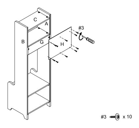
Step 7. Attach bottom back panel (part I) to assembled unit (parts A, B, F & G) using short screws (part #3) and phillips head screwdriver.
