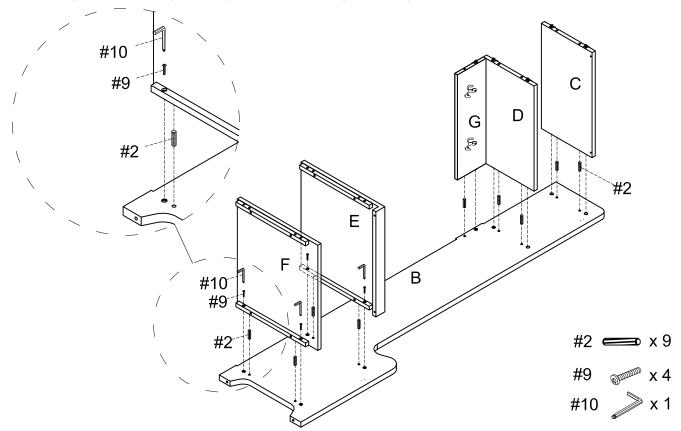
Step 5. Attach left side panel (part A) to assembled unit (parts C, D, E, F & G) using wood dowels (part #2), allen bolts (part #9), allen wrench (part #10) and lock the hardware.
